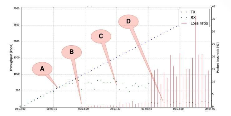
Point **A** indicates the area of initial saturation of the data link. Point **B** shows the moment of the first recorded loss of packet. Point **C** is in the area of maximum data link throughput before significant loss of packets begins. A heavily congested data link is the area around the **D** point.
