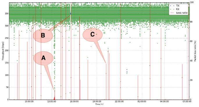
At point **A**, there is a deterioration in the data link transfer properties leading to a decrease in bit rate and accumulation of loss. Point **B** indicates a more serious problem of interrupting communication in a few tens of minutes. Packet loss at point **C** is a brief deterioration of data link parameters over a few seconds.
